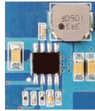
BD9D321EFJ PCB 17mm×20mm=340mm 2
